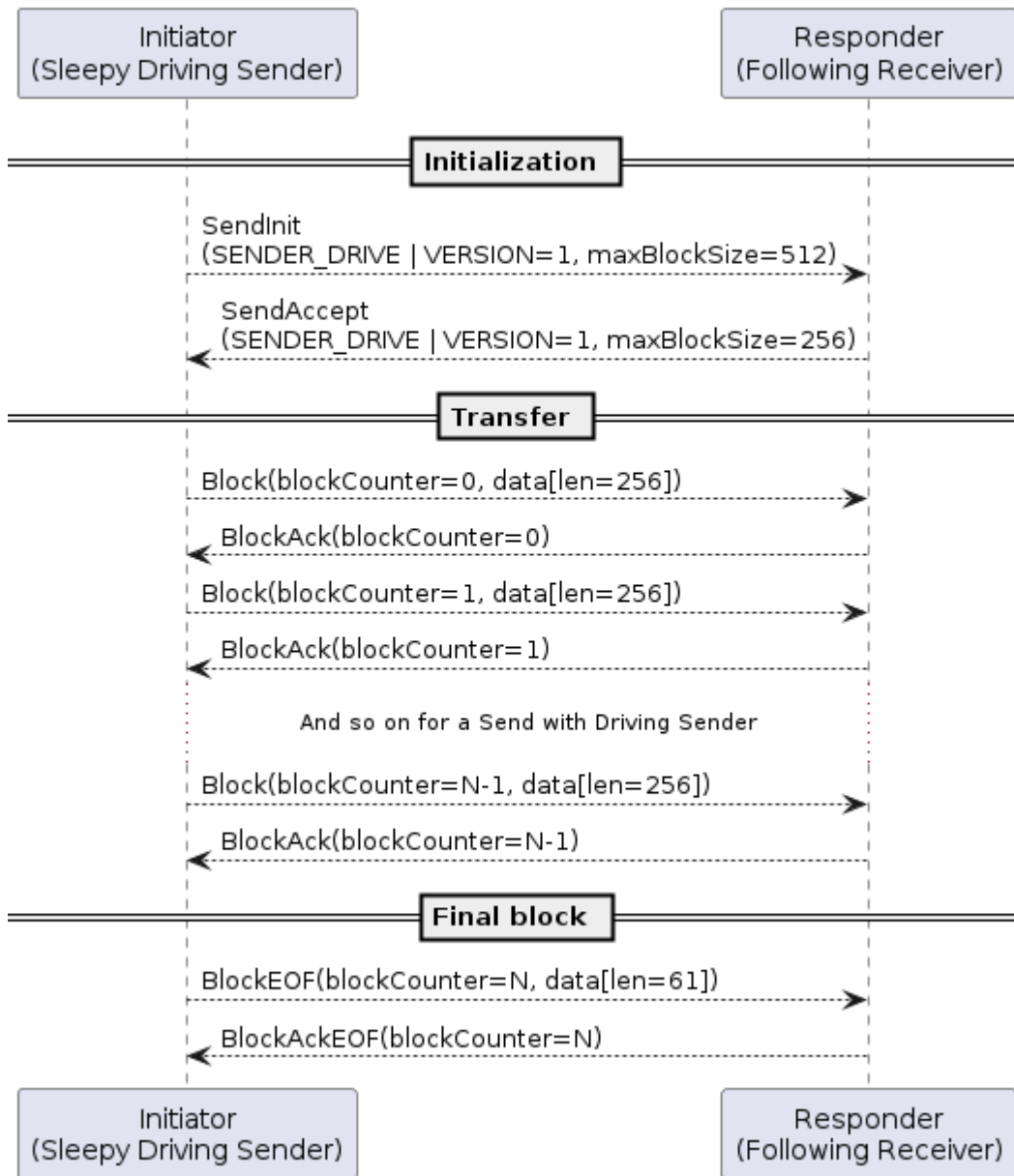
Figure 87. Synchronous file sending from sleepy device acting as driving Sender
