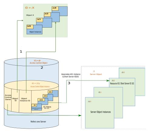
Figure: 8.1.2.2.-1 Illustration of the relations between the LwM2M Access Control Object and the other LwM2M Objects
