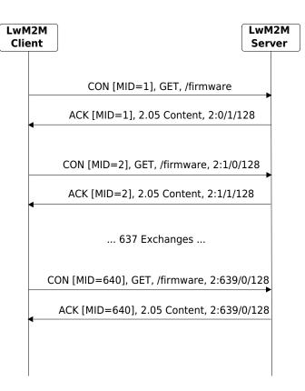
Figure: E.6.2-2 Example of a client fetching a firmware image
