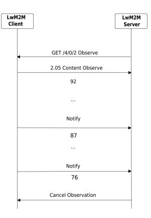
Figure: 6.4.–1 Example flow for Information Reporting Interface for the RSSI Resource of the Connectivity Monitoring Object of the example client Appendix LwM2M Objects defined by OMA (Normative)
