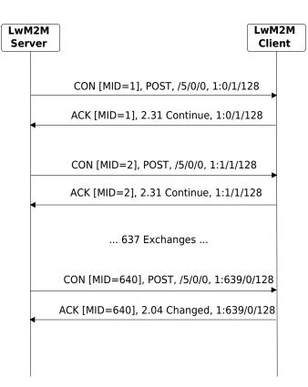
Figure: E.6.2-1 Example of a LwM2M Server pushing a firmware image to a LwM2M client
