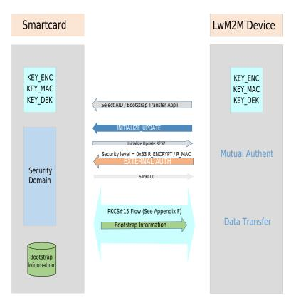
Figure: H.-1 Bootstrap Information transfer from Smartcard to LwM2M Device using Secure Channel according to [GLOBALPLATFORM]
