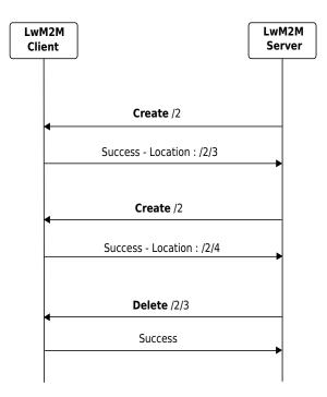
Figure: 6.3.-1 Example flows of Device Management & Service Enablement Interface
